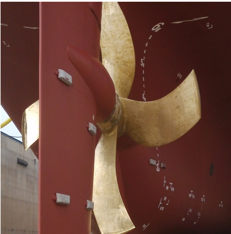
The CLT propeller installed on M/V JS GREENSTONE
